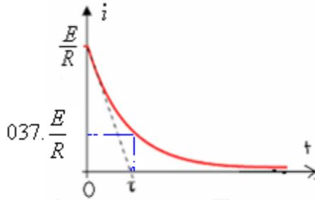
$$i = \frac{dq}{dt} = \frac{d(C u_c)}{dt} = C \frac{du_c}{dt} = C \frac{d[E(1 - e^{-\frac{t}{\tau}})]}{dt} = C \left[ \frac{E}{\tau} \right] e^{-\frac{t}{\tau}} = C \frac{E}{RC} e^{-\frac{t}{\tau}} = \frac{E}{R} e^{-\frac{t}{\tau}}$$
