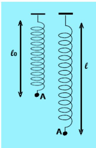
$$W_{A_0 \rightarrow A_2}(\vec{F}') = \int_{x_0}^{x_2} Kx dx = \frac{1}{2}K(x_2^2 - x_0^2) = K \frac{x_2^2}{2} = 6,5 \times 10^{-2} \text{ J} \quad - 2$$
